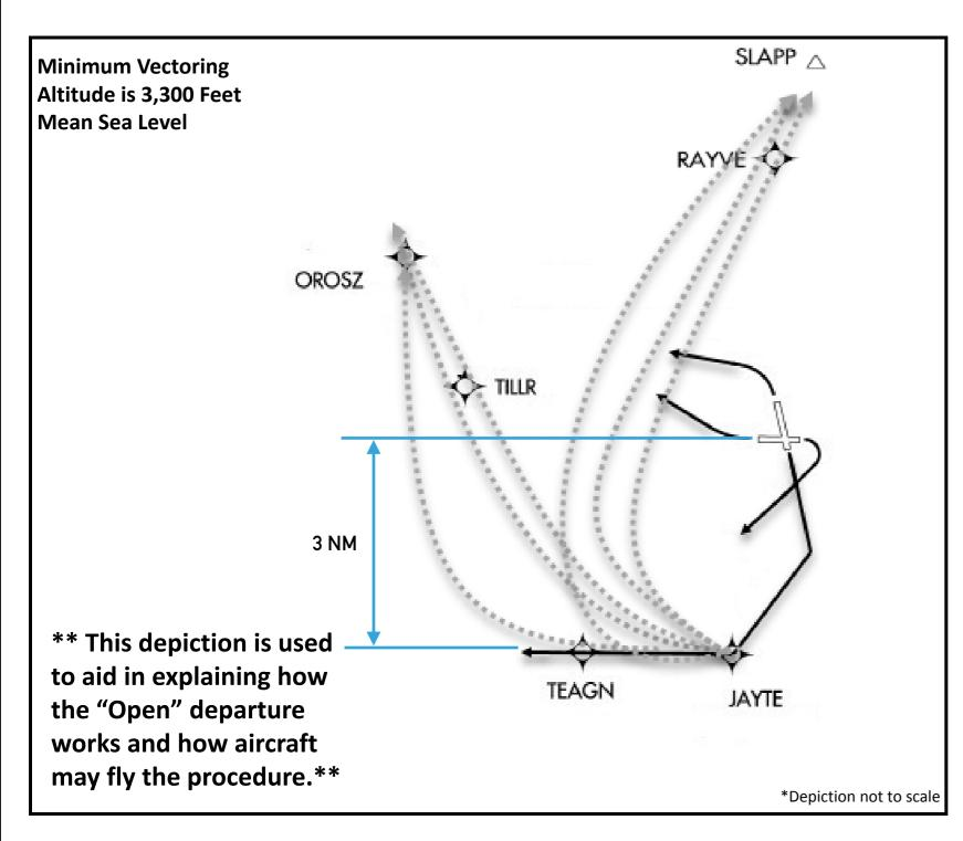
Because of the airspace complexity and congestion around Burbank, the FAA determined that Burbank would benefit from a new, hybrid departure route known as an "open" departure. An open departure begins with a satellite-based navigation segment, then transitions to a segment where air traffic controllers can dynamically maneuver aircraft through certain congested areas, and then connects with another satellite-based segment.
